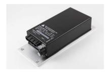
B62SR/B40SR/B70SRfamily provides single output voltages including 12.4V/13.5V output. With input range of 18-106Vin, B62 family converter delivers up to 300W output power. With input voltage range of 18 – 60V, B40SR family delivers up to 300W output power. With input voltage range of 36-106V, B70SR family delivers up to 300Woutput power. Typical efficiency of this compact size DC-DC is up to 89%.
